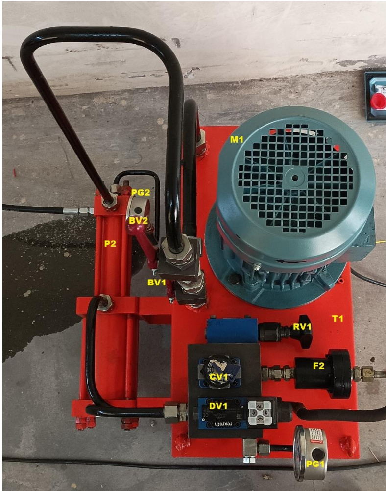
Top view of the Hydraulic Blade Holding System
