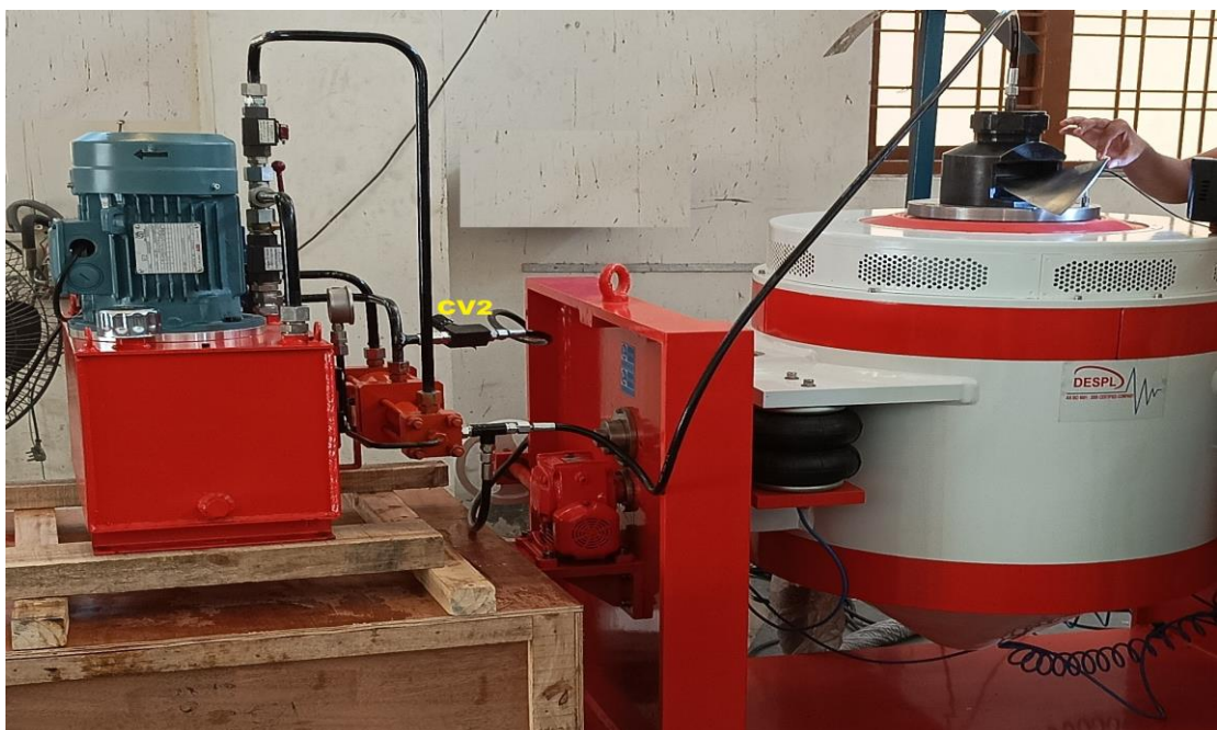
Pick of the Blade Holding Hydraulic System connected to the fixture
